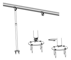
To park the leg in the front profile, turn the leg 90 degrees and lift it from the foot plate - fold the leg and click it in the snap bracket.
