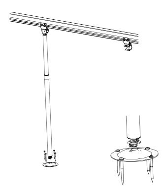
**To adjust the length:** Hold the lower profile of the leg and turn the upper profile to release the fixing - adjust to the desired length - turn the upper profile to stop.
