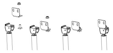
2. Assemble the snap-in brackets on the angle brackets.
