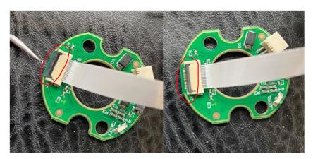
Step 4: Once tape is separated simply replace with new microchip board.
