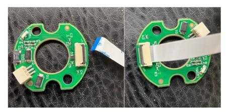
Step 5: Plug in the tape to the new board. NB: the black locking tab needs to be pushed in so the tape can insert properly. Once inserted pull the black tab to lock the tape in place.
