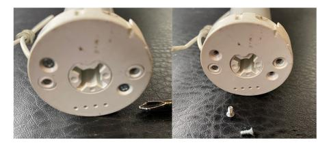
Step 2: Remove cover and pull-out chip board. NB: tape will be attached. Pull on this to extend.
