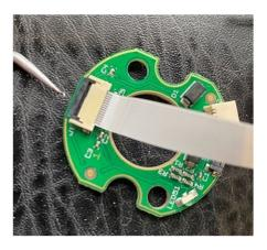
Step 6: Re assemble. NB: motor will need to be re coded.
