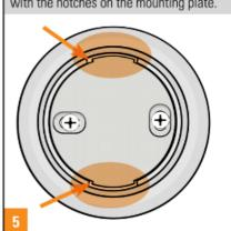
INSERT the Surface ring around mounting plate, ROTATING to the right to securely lock into place.
