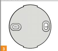
ATTACH the Surface mounting plate to the mounting surface using the screws provided.
