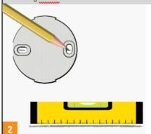
Use the screw holes on the Surface mounting plate to mark the location. The Hunter Douglas logo should appear right side up and be horizontal.
