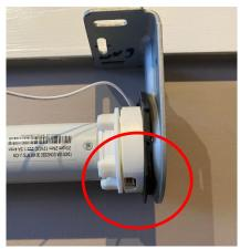
If you choose to have the motor on the left, the charger port will be difficult to access so you will need to rotate the adapter at the end of the motor head. For this change, you will require a T20 star Head bit to unscrew screws from plate.
