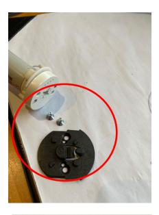
Step 2 - Turn the adapter 90 degrees and screw back into place
