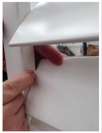
6. With a small Hammer and Punch, gently tap the replacement control pin through the center control rod into the louvre.
