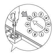
Set the motion threshold adjuster to between 3-6.
