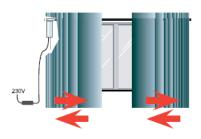
Press Up button on the remote. The motor will begin to learn end limits. Don't stop the motor until the end limits have been reached and the motor has completely stopped.
