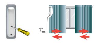
Briefly press the program button on the remote. The motor will jiggle and the remote has been recorded.
