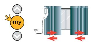
To reverse the motors direction, press and hold the **my** button for more than 5 seconds. The motor will jiggle.
