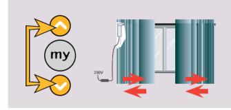
Press and hold the Up and Down buttons on the remote for 2 seconds. The motor will jiggle.
