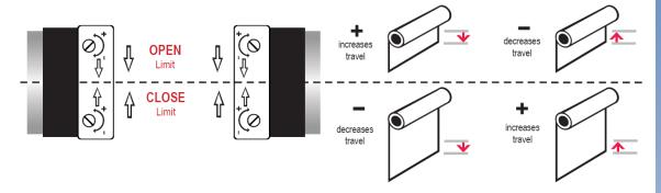
Limit settings can be adjusted using a limit setting tool, hex key or flat head screwdriver. Power must be supplied to the motor in the direction required in order to set the limits. Turn the limit screws in the direction indicated above to increase or decrease blind travel.
