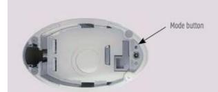
Press and hold the Mode button until the Green LED turns off.
