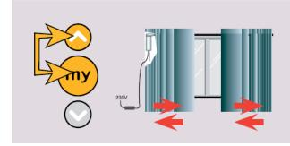
Press and hold Up and **my** buttons until the motor jiggles. The curtain will continuously open and close.
