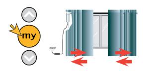
Press and hold the **my** button until the curtain jiggles. The new speed has been confirmed.
