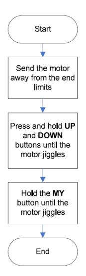
Before changing the motor rotation direction, the motor must be completely programmed with a remote
