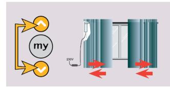
Press and hold the Up and Down buttons until the curtain jiggles.
