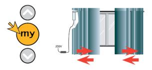
Press and hold the **my** button until the curtain jiggles. The curtain direction has been changed.
