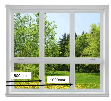
Example: Window Reveal width is 1500 with two T-Posts. 1<sup>st</sup> T-Post at 500mm 2<sup>nd</sup> T-Post at 1000mm
