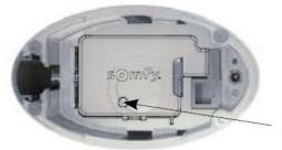
Program button Using a paperclip, press and hold the program button for 12 seconds.
