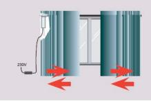
The motor will jiggle 3 times. The motor memory is erased.
