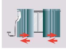
The curtain will jog 3 times. The memory of the motor is erased. If power is maintained to the motor, it will automatically learn new limits.
