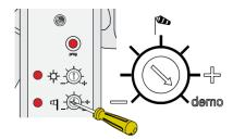
Set the sensor into demo mode by turning the wind adjuster to 'demo'
