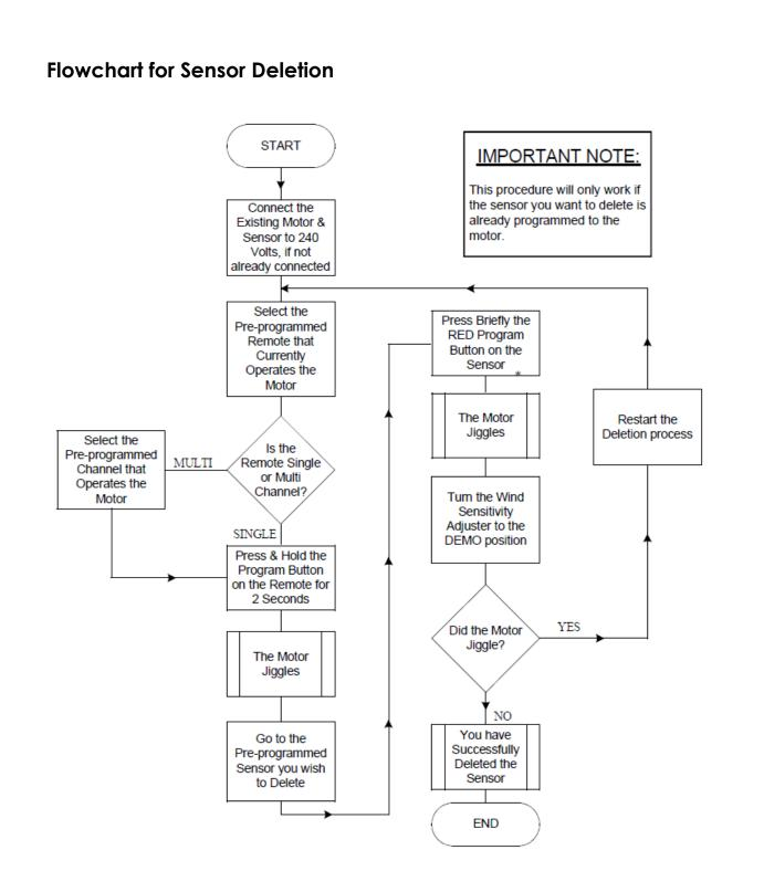
**Note:** Keep pressing the program button until the motor jiggles twice to delete all sensors
