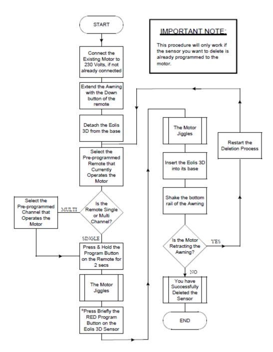
**Note:** Keep pressing the program button until the motor jiggles twice if you wish to delete all sensors.
