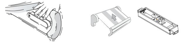
Test the sensor functionality by shaking the awning. The awning shouldn't retract if the sensor has been deleted correctly. sensor deleted
