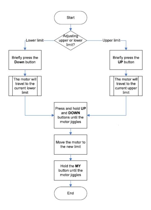
Before adjusting end limit, the motor must be completely programmed with a remote.
