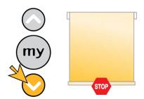
Briefly press the Down button, and the motor will travel to the current lower limit.
